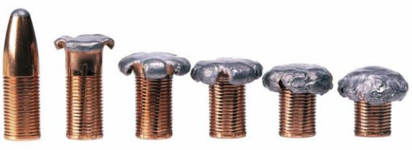
North Fork .416 caliber, 370 gr bullets recovered at progressively higher impact velocities. 1735 f.p.s. / 99.5% retention; 2000 f.p.s. / 99.4%; 2200 f.p.s. / 99.3%; 2400 f.p.s. / 97.8%; 2600 f.p.s. / 95.0%. The core bonding process achieves 95% weight retention even at 2600 f.p.s. impact velocity.
